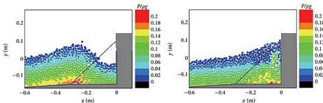
**Figure 44:** Model for the impact of storm waves on a permeable structure (Pu & Shao, 2012).
