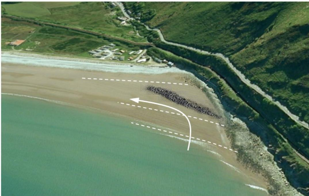
**Figure 35:** Proposed artificial reef to deflect storm waves at Friog corner.
