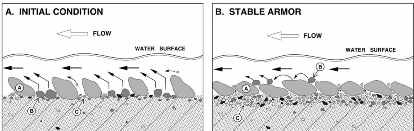
**Figure 45:** Mechanism by which the upper surface of the storm beach may become armoured against wave erosion (Hayes, Michel, & Betenbaugh, 2010).
