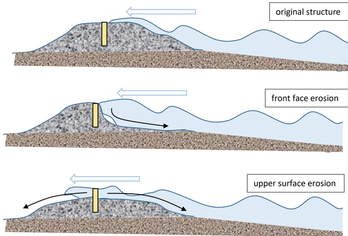
**Figure 43:** Conceivable mechanisms by which a breach of the shingle spit could occur.
